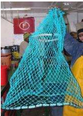
Figure 25: Cetacean exclusion device (CED) mad up from trawl net.
