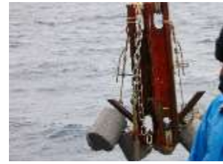
Figure 8: Steel anchor used to anchor end of the longline. Note also concrete weights.
