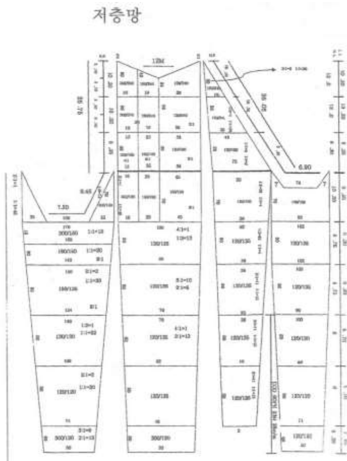
Figure 2: Drawing of the Custom Manufactured Bottom Trawl Net of the vessel1.
