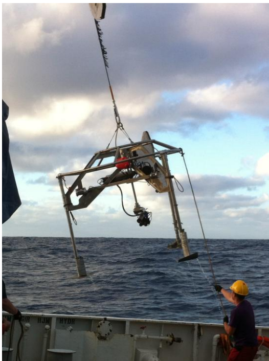
Figure 4. The CAMPOD towed video rig being launched from the RV Dr Fridtjof Nansen.
